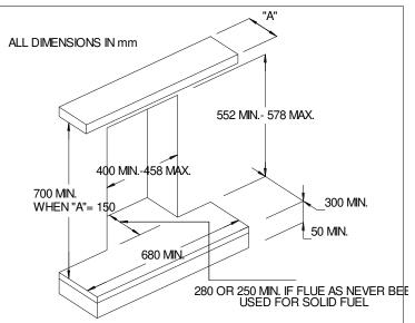
thickness of the spacer must be added to the minimum 300mm hearth depth to comply with regulations.
