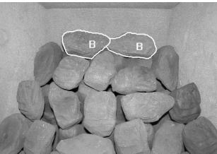
• Add the final 2 x B and 1 x A coals as shown to the top of the coal bed. Arrange so as to be stable. The layout is now finished.
