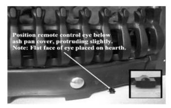
Check that a signal is being received by pointing the remote control hand set in the direction of the appliance and simultaneously press the buttons marked <sup>(1)</sup> and 'standby'. Continue to hold in these two buttons until a 'bleep' is heard (approximately 2-3 sec.). If no sound is hear check position of remote control eye.
