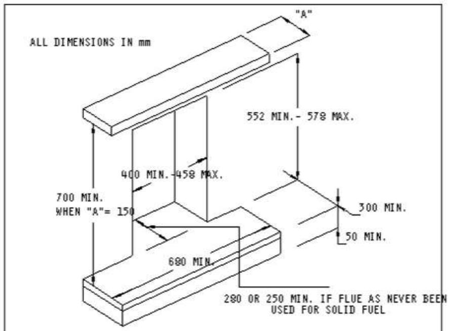
Any permanent flue restriction or variable dampers are to be removed or locked fully open. The chimney should be swept prior to installation if not new.
