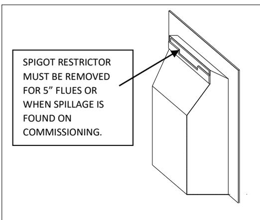
**Note:** Dampers or register plates must not restrict any of the above flues. The flue must only service a single appliance and not have any branches or traps, which may impede the natural draught. If a terminal is fitted it must be suitable for the purpose.
