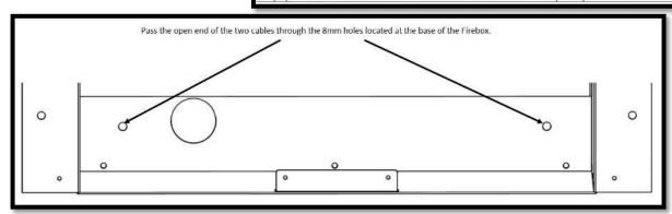
Fix the fire casing back into the opening using the cable fixing system as shown in do not cut off loose ends of cable after fixing, coil and tuck carefully behind burner tray.
