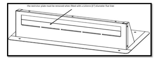
IMPORTANT: - the restrictor plate must be snapped off from the flue adptor when the appliance is installed into this type of flue.
