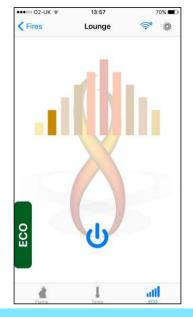
In **ECO** mode the flame height will automatically be adjusted up and down.
