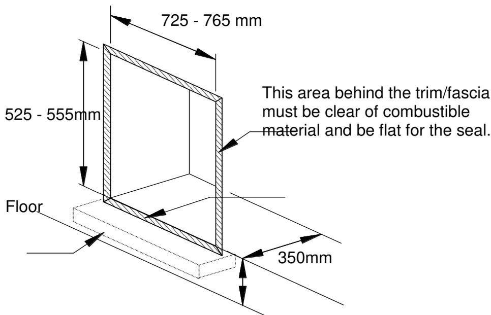
The front face and the base of the fire opening must be flat to ensure that a good seal is formed between the rear and base of the appliance and the chimney to avoid any reduction of natural draught. \* **Please note: It is important to ensure the bottom of the firebox is completely sealed to reduce the risk of excess sooting resulting from incomplete combustion.**
