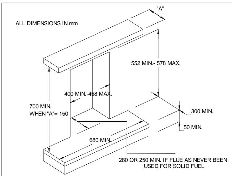
Fireplace opening must be 552 mm - 578 mm high by 400 mm – 435 mm wide (or up to 458 mm if the cable fixing system is used).
