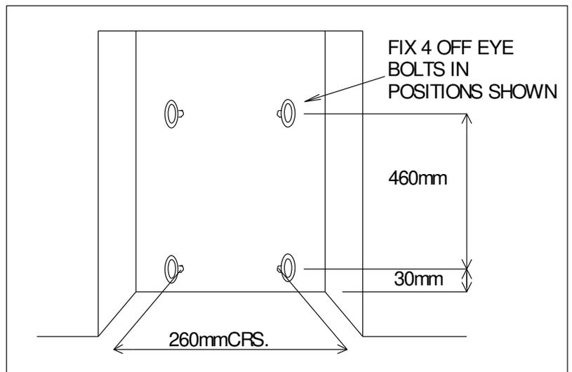
Fix the fire casing back into the opening using the cable fixing system as shown in do not cut off loose ends of cable after fixing, coil and tuck carefully behind sides of Refractory back
