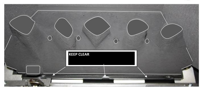
• When positioning the rear matrix be careful not to cover the burner ports
