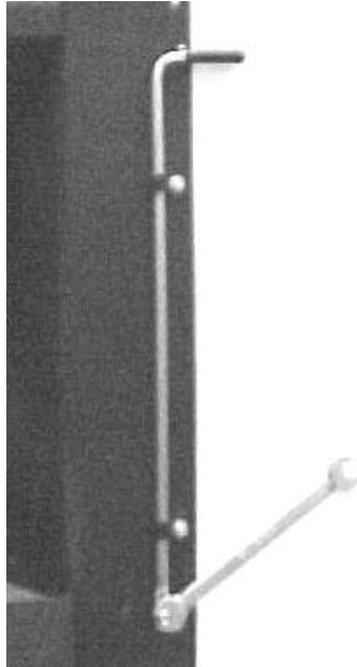
Flip the slide control lever round so that the rubber-capped end is protruding out to the right as shown in the left-hand picture. Check that it slides freely up and down in the nylon slide guides. Remove the nylock nut with a 7mm A/F spanner as shown
