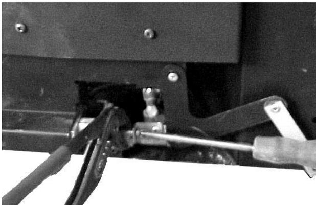
Taking great care grip the copper protective sleeve at the end of the gas control spindle (DO NOT GRIP SPINDLE IN AND OTHER PLACE) as shown and remove the screw from the end as shown above.
