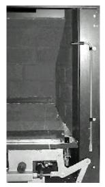
Flip the slide control lever round so that the rubber-capped end is protruding out to the right as shown in the left-hand picture. Check that it slides freely up and down in the nylon slide guides. Remove the nyloc nut with a 7mm A/F spanner as shown.
