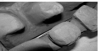
Place the first row of 3 x A and 3 x B overlay loose coals as shown between the front coals and base matrix. Make sure that they are stable and DO NOT let them fall down in the gaps between the peaks on the matrix.
