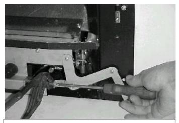
Taking great care grip the copper protective sleeve at the end of the gas control spindle (DO NOT GRIP SPINDLE IN ANY OTHER PLACE) as shown and remove the screw from the end as shown above.
