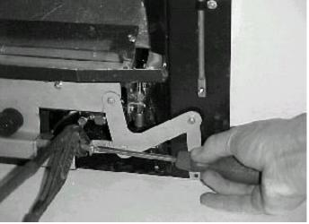
Check for gas soundness. Reconnect the bell crank mechanism as above ensuring that the gas control spindle is gripped only over the protective copper sleeve and no other part of the spindle as, ensure NO side strain is applied to the spindle.
