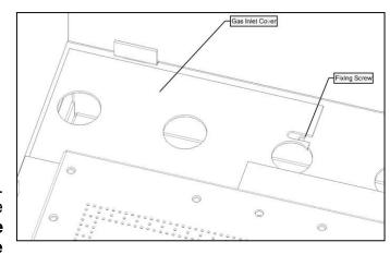
inlet cover retaining screws and nut should be fitted from the rear of the firebox flange at this stage. The required fixing can be found within the fireplace frame packaging
