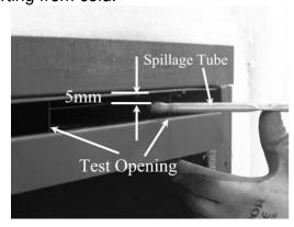
If spillage is detected the cause must be discovered and the fault corrected, if the fault cannot be corrected, disconnect the fire from the gas supply and seek expert advice. Spillage can be caused
