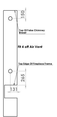
• Fit the four off 70mm diameter circular soffit vents provided with the appliance.
