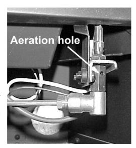
Note: - Take care when cleaning in this area so as not to damage the pilot assembly.
