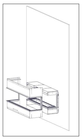
Place a further piece of 10mm heat resistant board 956mm x 258mm within the false chimney fascia.
