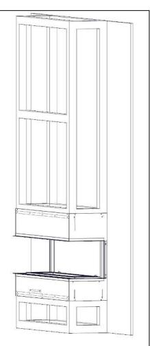
Using suitable board and fixing, cover both side and front sections of the false chimney.
