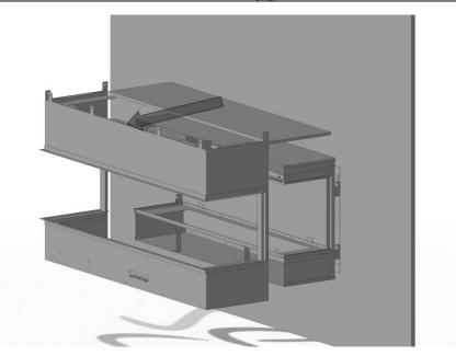
Why supporting the fascia, slide the EDB unit over the 3mm stud located on the bottom rear channel face. Retain the unit using the M3 nut and washer provided.
