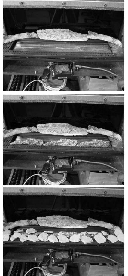
Place three shapes shown within the burner top plate and air tray as shown.
