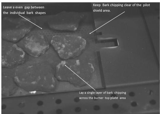
Place the 2 log shapes along the front edge of the burner top plate. Place a single layer of small bark chippings along the rear of the burner plate. (Please note vermiculite will be provided on LPG models)
