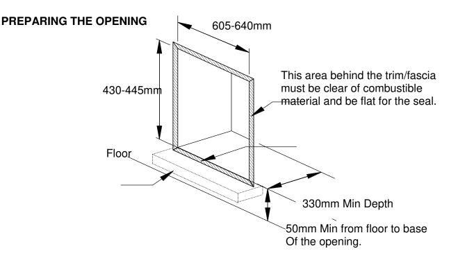
The front face and the base of the fire opening must be flat to ensure that a good seal is formed between the rear and base of the appliance and the chimney to avoid any reduction of natural draught.
