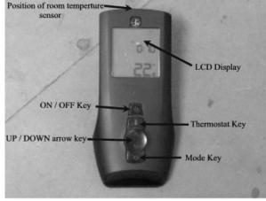
c. With the appliance lit, by pressing key the operational mode is switched from manual to Room thermostat setting and vice versa. When Room thermostat mode is active, the display shows the
