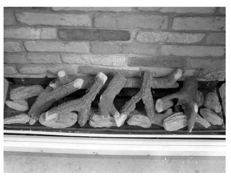
• Place the last Two large shapes LH and RH as shown.
