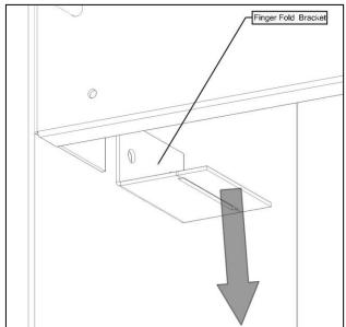
With the two rear liner in position. Offer the LH and RH side liner into the bottom brackets within the burner Shelf assembly. (Please note the patterned edge must be positioned along the front). Push the top of the liner back into the chamber sides and bend the finger fold brackets to locate the side liners.
