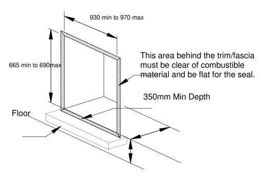
The front face and the base of the fire opening must be flat to ensure that a good seal is formed between the rear and base of the appliance and the chimney to avoid any reduction of natural draught. \* Please note: It is important to ensure the bottom of the firebox is completely sealed to reduce the risk of excess sooting resulting from incomplete combustion.
